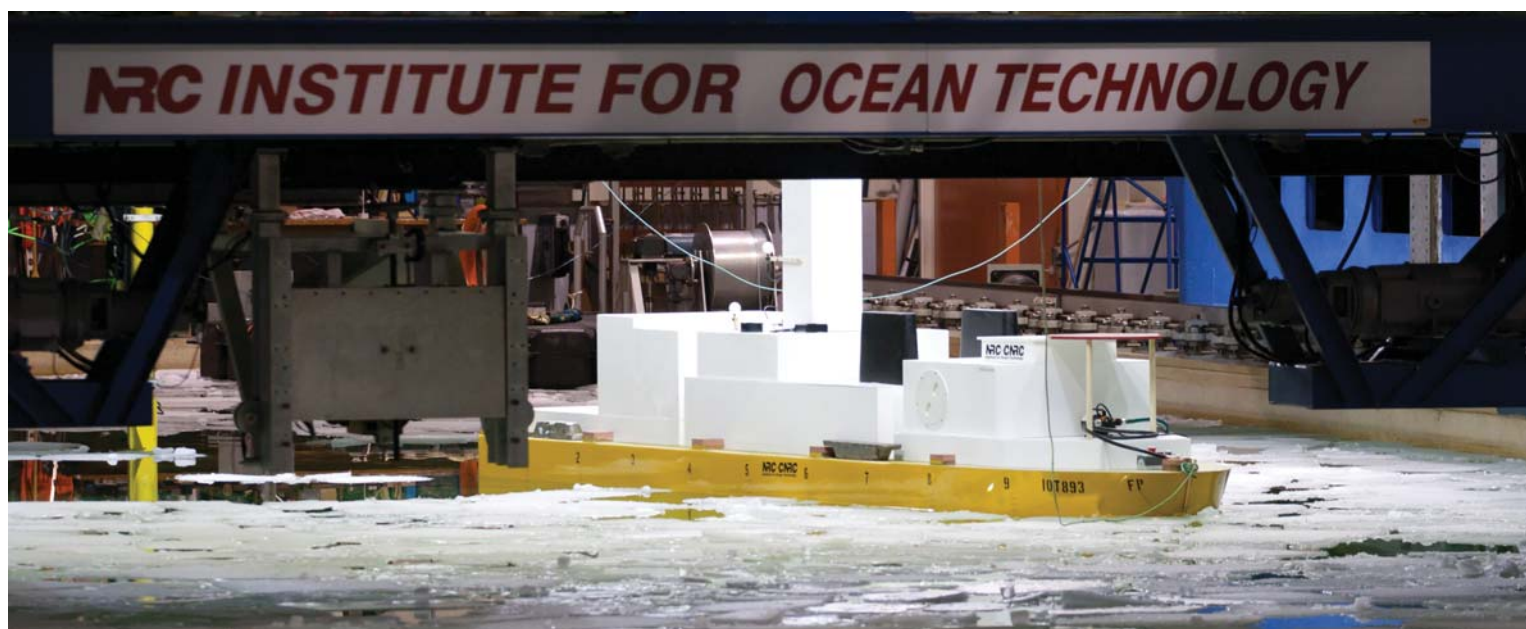
Generic model of a drillship during a DP experiment in ice.
