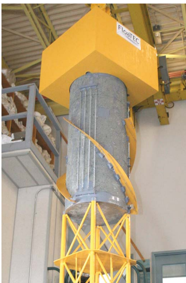
Spar model with belly strakes.
