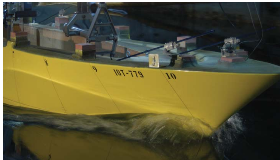
Model during calm water resistance test.
