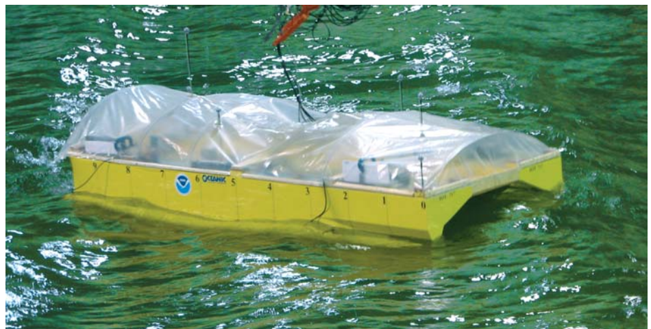
SWATH model during a zero-speed seakeeping test.
