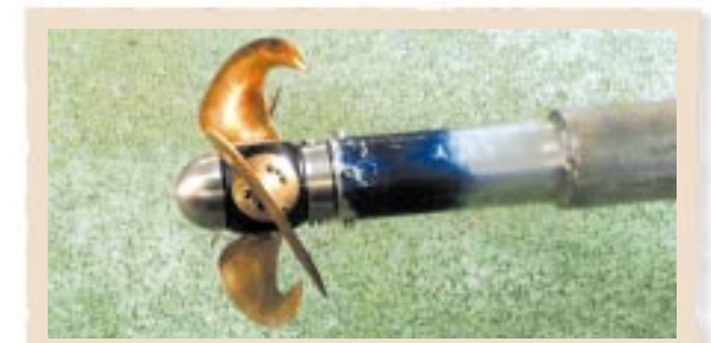
▲ Highly-skewed propeller on new dynamometer tested in IMD ice tank
