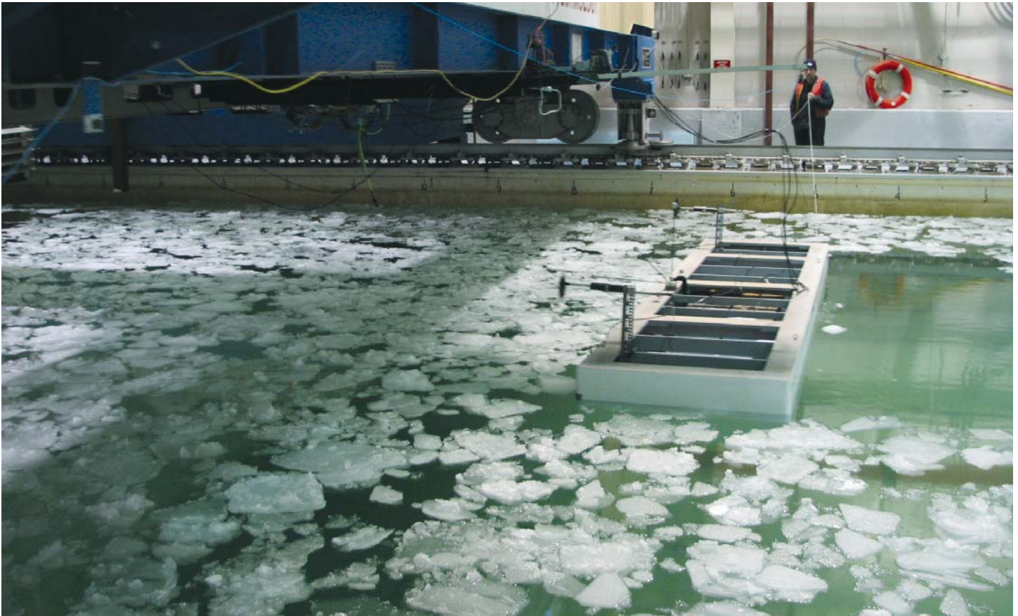
Illustration of the exposed channel created behind the barge in the 90-meter Ice Tank.
